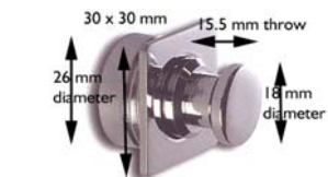
Drill hole 26 mm diameter for ring
