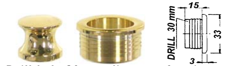
Drill hole 30 mm diameter for ring
