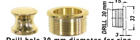
Drill hole 30 mm diameter for ring
